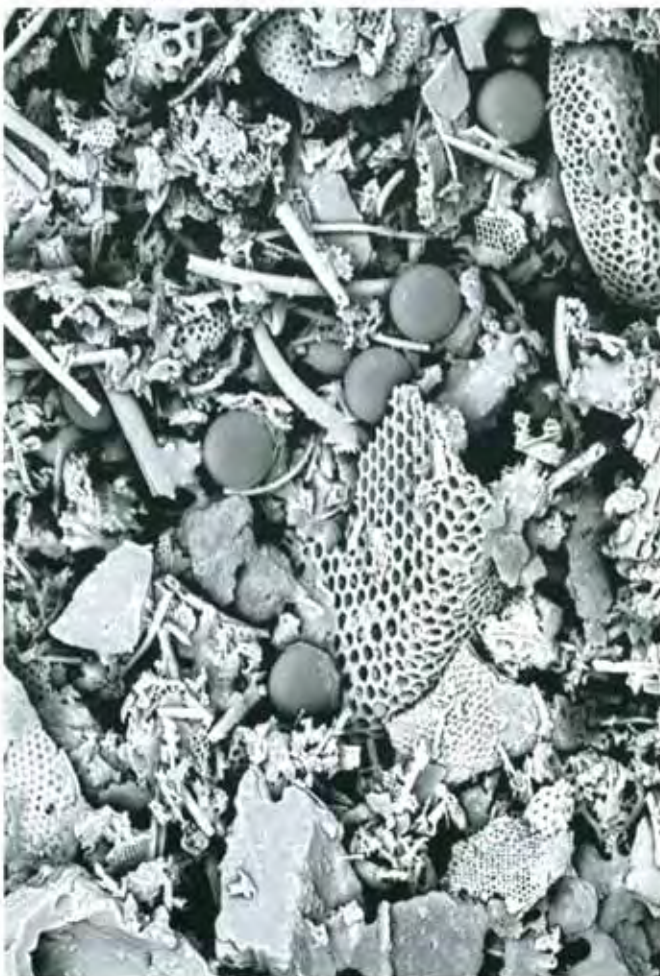
Scanning electron micrograph of 10µ latex beads in a cake of Hyflo® Super-Cel® (1000x)
